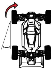
By turning the steering wheel to the left the model steers to the left. Turning to the right also steers the model to the right.
